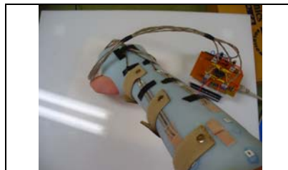
Figure 10: Cast worn by Blum, connected to DAQ (Blum, 2007)
