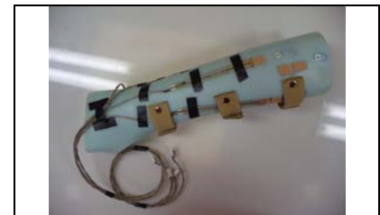
Figure 11: Cast with sensors mounted (Blum, 2007)
