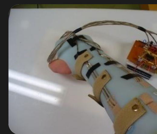
Figure 10: Cast fully equipped with sensors mounted (Blum, 2007)
