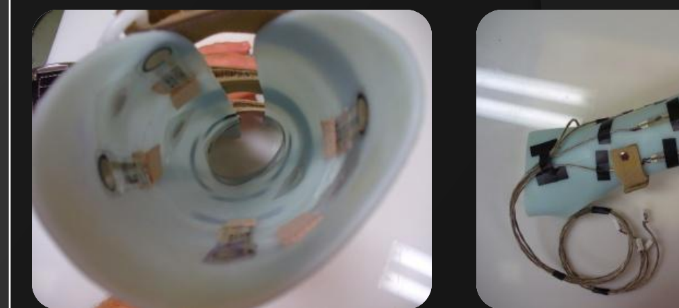
Figure 9: Internally mounted force sensors (Blum, 2007)
