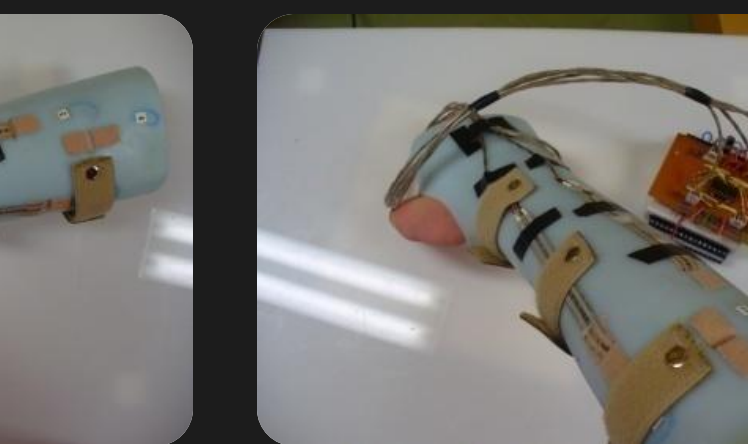
Figure 10: Cast fully equipped with sensors mounted (Blum, 2007)
