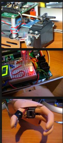
Figure 11 (a-c): (From top) Servo actuator and vibration amplification circuit board; LED # Force Readout (scale of 0-6) + Vibration Warning LED; hand with vibration sensor (Blum, 2007)
