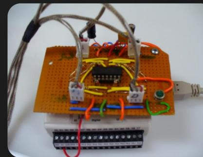
Figure 10: DAQ and amplification circuit board with four force sensors connected (Blum, 2007)
