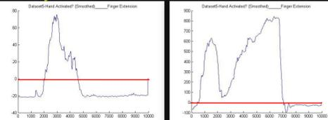
Figure 14(a & b): Myoelectric and Force Sensor Finger Extension Smoothed SVEN Function (Blum, 2007)
