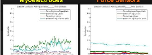
Figure 13(a & b): Comparison of Wrist Extension Raw Calibration Data (Blum, 2007)
