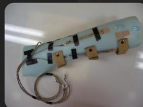
Figure 8: Cast fully equipped with sensors mounted (Blum, 2007)
