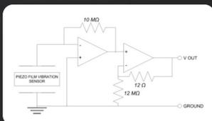
Figure 3: Vibration Sensor Circuit (Kyberd/Blum, 2007)
