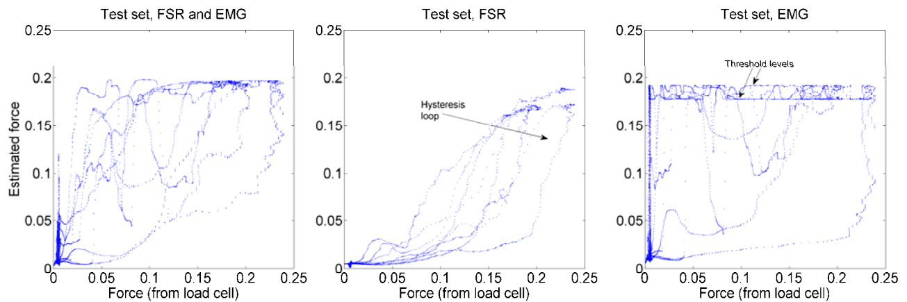
Fig. 4: Measured vs estimated force using an MLP with 4 hidden nodes. Same data set as in Fig. 3.
